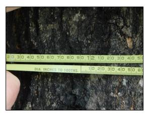
The tape is placed around a standing tree as shown in the picture. This tree is 11.9 inches in diameter. In most cases, the measurement is rounded off to two-inch classes, such as 10, 12, 14, 16, etc. This tree would be tallied as a 12 inch tree.
