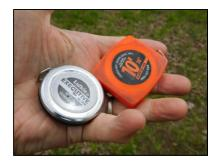
Here are two diameter tapes manufactured by different companies. As you can see, they are very small and easy to carry in a pocket. These tapes (called D-tapes), are used by foresters and technicians when cruising timber.
