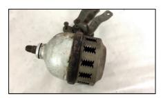
The object in the last issue is a bicycle siren. It was mounted on the bicycle frame at the front wheel. A chain was attached to it that reached to the handle bar of the bicycle. When the chain was pulled, the round tip of the siren was pulled against the front wheel which produced the sound of a siren. There was a long hill near our house. I would ride down that hill (which was gravel at that time)
