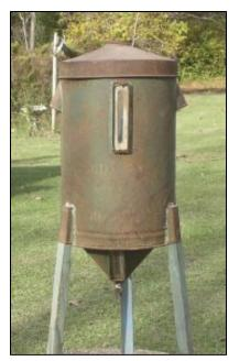
Left: -- Gravity Type Cream Separator. We had this at our farm, but I never saw it being used. As I understand it, you could look through the glass on the side to see when the cream rose to the top and there is a spigot at the bottom.
