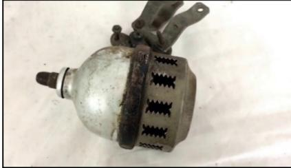
The object in the last issue is a bicycle siren. It was mounted on the bicycle frame at the front wheel. A chain was attached to it that reached to the handle bar of the bicycle. When the chain was pulled, the round tip of the siren was pulled against the front wheel which produced the sound of a siren. There was a long hill near our house. I would ride down that hill (which was gravel at that time)
